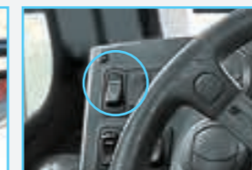
Screen Changeover Switch
