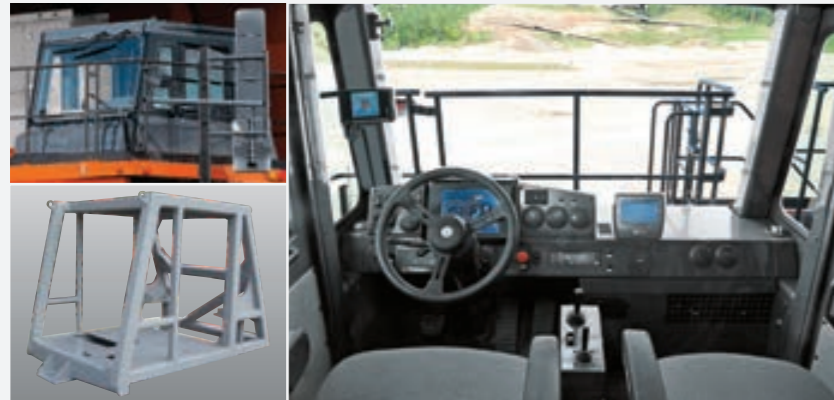
Note: This image shows a monitor for optional SkyAngle at the left pillar.
